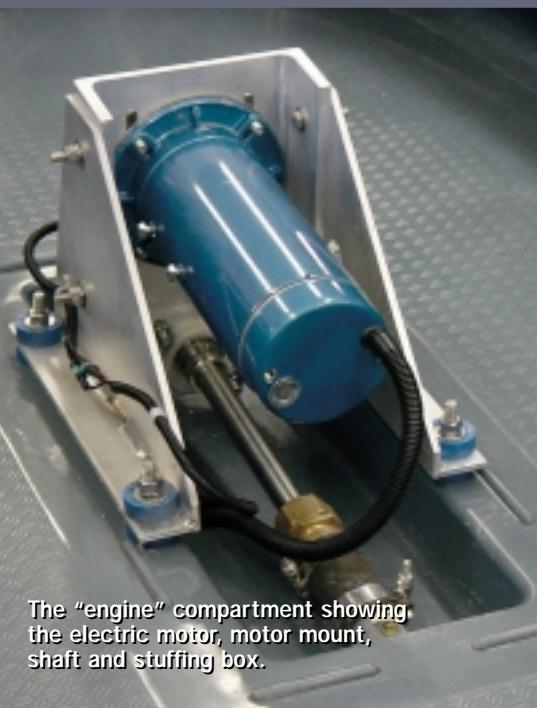
The "engine" compartment showing the electric motor, motor mount, shaft and stuffing box.
